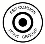
This symbol is established to indicate an ESD common point ground, which is defined by ANSI/ESD-S6.1 as "a grounded device where two or more conductors are bonded."
